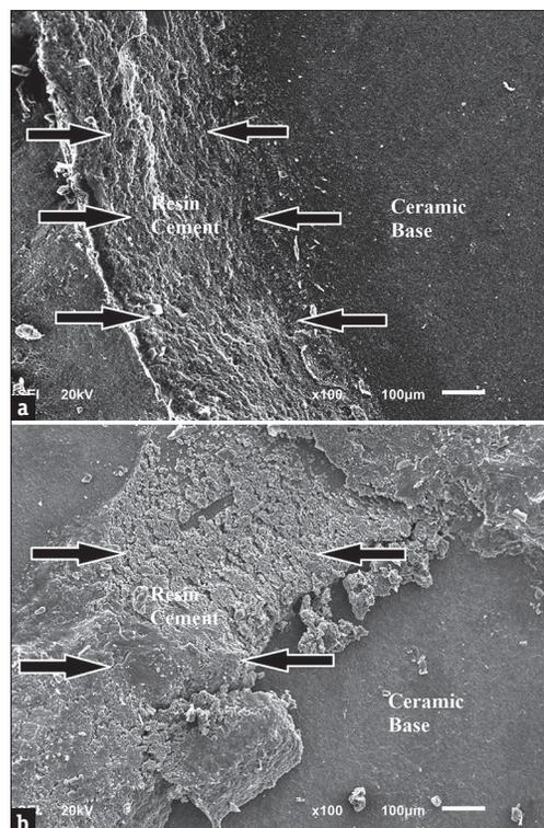
**Figure 3:**(a) Scanning electron microscopy image of Group S (silica coating) after debonding; mix fracture, (b) SEM image of Group SL1 (silica coating+laser 1) after debonding; mix fracture
