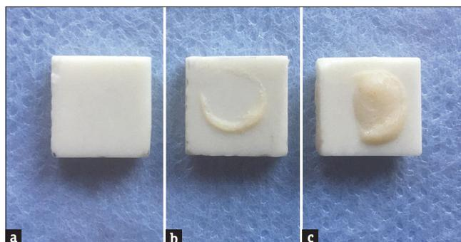
**Figure 2:** The images of failure types; (a) adhesive, (b) mix, (c) cohesive
