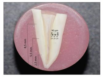
Figure 1: Nano-indentaion measurement points at three regions from root canal lument to cementum
