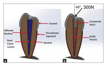
**Figure 2:** The structures, materials, and the loading conditions of the FEA models. (a) The unfilled model and (b) the model assumed to be filled with gutta-percha and restored using composite resin
