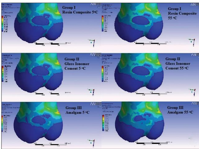
Figure 5: The distribution of von Mises stress according to groups
