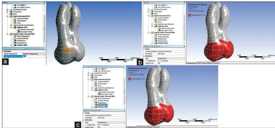
Figure 4: (a) The base temperature (36.5°C). (b) First thermal load (5°C). (c) Second thermal load (55°C)
