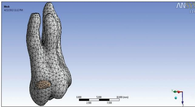
Figure 2: The meshed model
