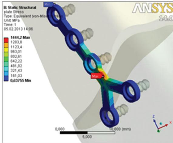
**Figure 7:** Three-dimensional von Mises stress distribution fields in the Y plate
