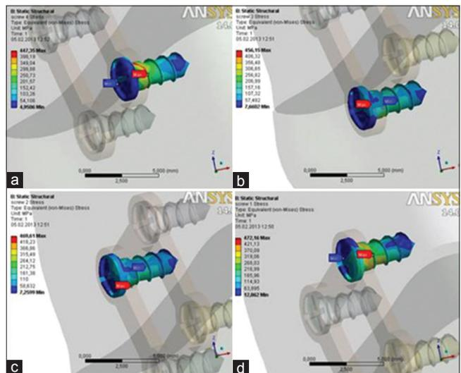
**Figure 6:** Three-dimensional von Mises stress distribution fields in screws of the square plate: (a) 1<sup>st</sup> screw (b) 2<sup>nd</sup> screw (c) 3<sup>rd</sup> screw (d) 4<sup>th</sup> screw
