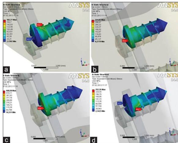
**Figure 3:** Three-dimensional von Mises stress distribution fields in screws of the upper plate: (a) 1<sup>st</sup> screw, (b) 2<sup>nd</sup> screw, (c) 3<sup>rd</sup> screw, and (d) 4<sup>th</sup> screw
