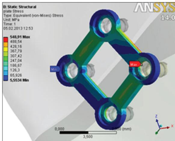
**Figure 5:** Three-dimensional von Mises stress distribution fields in the square plate
