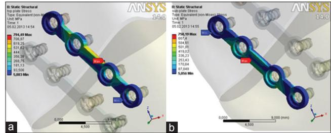
**Figure 2:** Three-dimensional von Mises stress distribution fields in (a) upper and (b) lower straight plate
