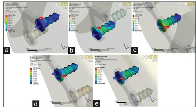
**Figure 8:** Three-dimensional von Mises stress distribution fields in screws of the Y plate: (a) 1<sup>st</sup> screw, (b) 2<sup>nd</sup> screw, (c) 3<sup>rd</sup> screw, (d) 4<sup>th</sup> screw, and (e) 5<sup>th</sup> screw
