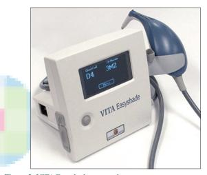
Figure 2: VITA Easyshade spectrophotometer
