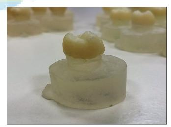
Figure 1: Prepared sample with orientation groove in the base
