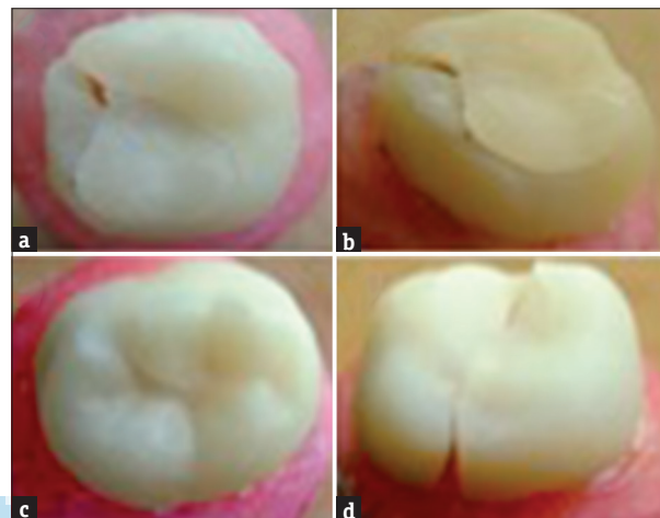
Figure 5: Crowns demonstrating score 2 failure types; Lava Ultimate (a and b), Vita computer-aided design-Temp (c), and Telio computer-aided design (d) (×10)
