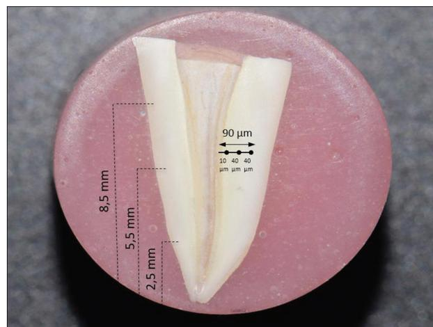
**Figure 1:** Nano-indentation measurement points at three regions from root canal lumen to cementum
