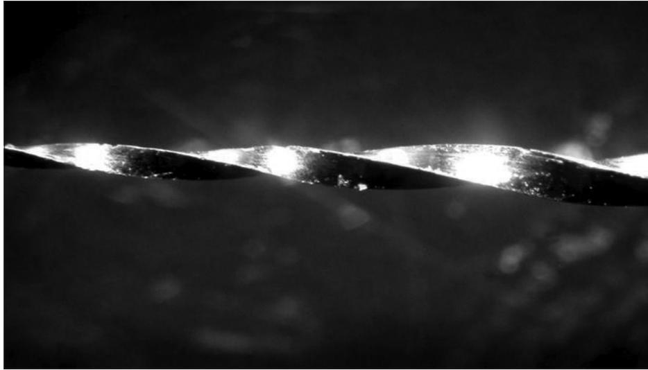
**Figure 3:** Deformation of EndoWave
