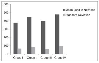
Graph 1: Fracture loads of teeth in four groups: Mean and standard deviation
