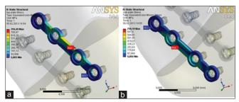
Figure 2: Three-dimensional von Mises stress distribution fields in (a) upper and (b) lower straight plate
