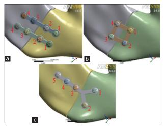
Figure 1: Three-dimensional finite element models: (a) Double straight plates; (b) square plate; (c) Y plate
