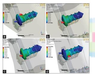
**Figure 3:** Three-dimensional von Mises stress distribution fields in screws of the upper plate: (a) 1<sup>st</sup> screw, (b) 2<sup>nd</sup> screw, (c) 3<sup>rd</sup> screw, and (d) 4<sup>th</sup> screw
