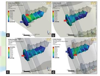
Figure 4: Three-dimensional von Mises stress distribution fields in screws of the lower plate: (a) 1<sup>st</sup> screw, (b) 2<sup>nd</sup> screw, (c) 3<sup>rd</sup> screw, and (d) 4<sup>th</sup> screw
