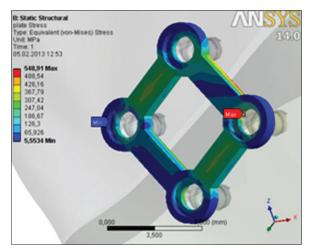
Figure 5: Three-dimensional von Mises stress distribution fields in the square plate
