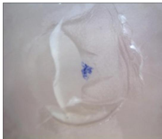
Figure 3: Cohesive fracture ( $\times 12.5$ )
