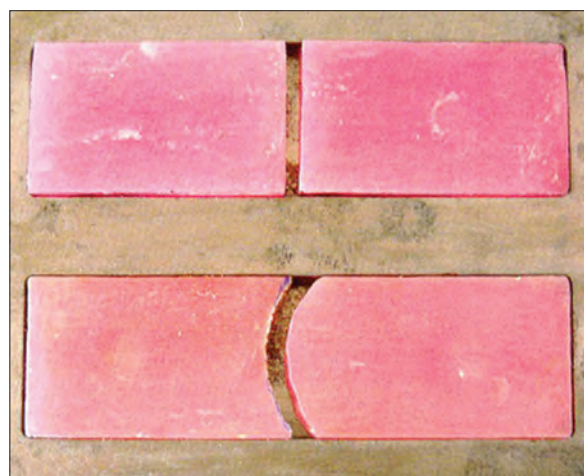
Figure 5: Mould 2 mm bigger than the original specimen in round and butt joint
