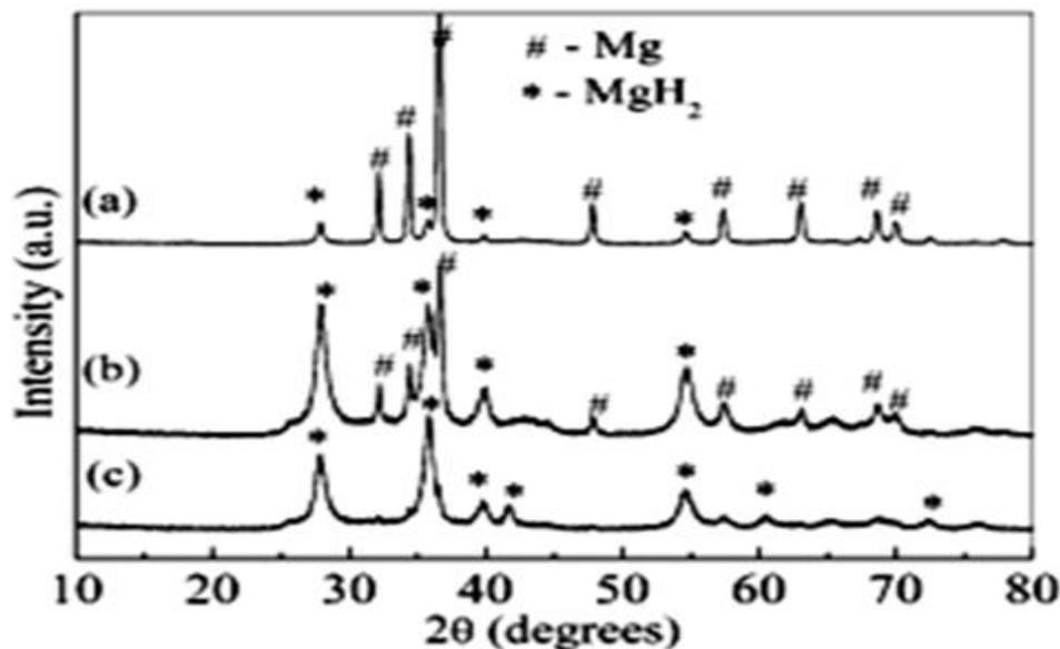
Figure 1: XRD Pattern showing peaks corresponding to magnesium and its hydride
