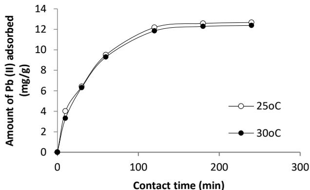
**Fig. 14. Rate curves Pb (II) Adsorption onto CVSS at Different Temperatures**
