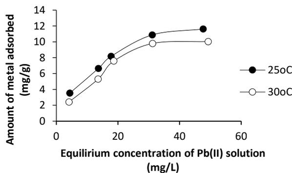
**Fig. 4 Isotherm Profiles for Adsorption of Pb (II) onto CVSS at Different Temperatures**
