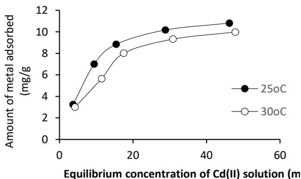
**Fig. 5 Isotherm Profiles for Adsorption of Cd(II) onto CVSS at Different Temperatures**
