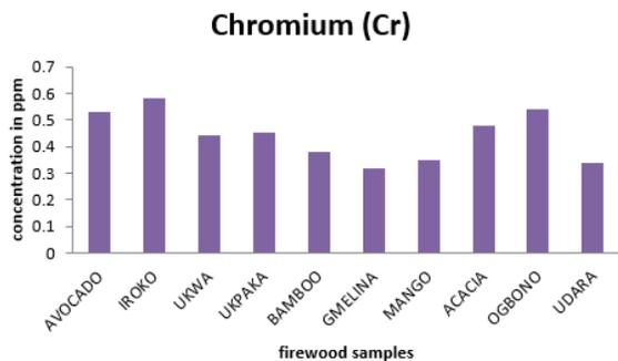
**Figure 10** A plot of Chromium in wood sample ash
