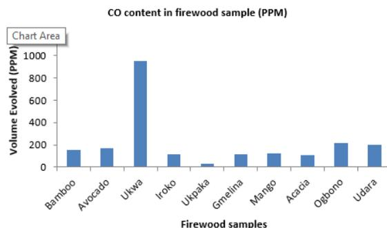
**Figure 3: Plot of CO content of the firewood samples.**
