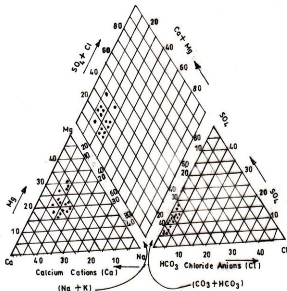
**Fig. 2:** Plots of Piper trilinear diagram for ground water in the Galambi area. (After Piper, 1944)
