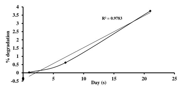
Figure 1: Variation of % degradation with days of a fixed weight of raw clay
