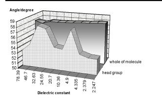
**Fig. 2:** A comparison of the variation of  $\theta_4$  dihedral angle degree, between DPPC head group and whole of the molecule.
