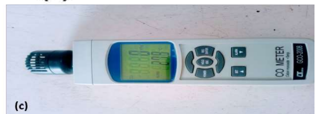
Fig. 2 Five Tons Press Type Briquetting Machine (a), Oxygen Bomb Calorimeter (GDY-1A) Set-up (b), Carbon Monoxide Meter (GCO-2008) (c). Production of typha grass fuel briquettes
