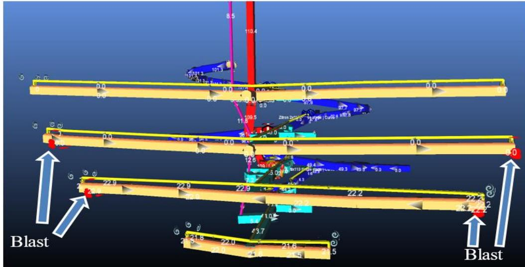
Figure 7: Two Ore Drives with Double Heading Blast Each
