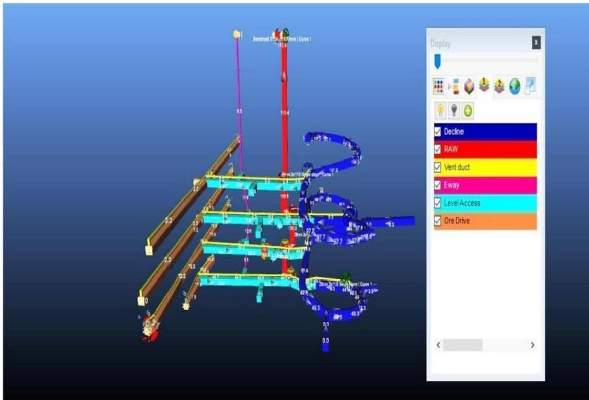
Figure 4: Ventilation Modelling of Underground Development at the Paboase Mine
