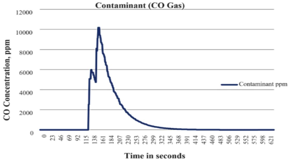
Figure 12: A Graph of CO concentration in ppm against Time in seconds (Scenario 2)
