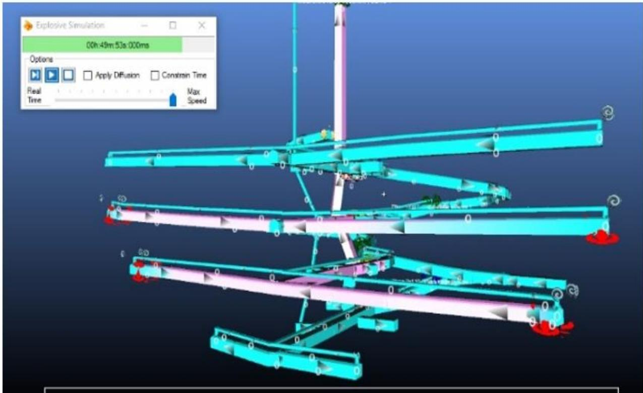
Figure 13: Ore Drives with Single Heading Blast Simulation
