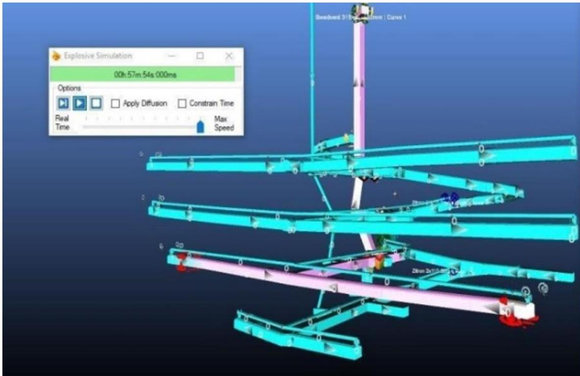
Figure 11: Double Heading Blast Simulation
