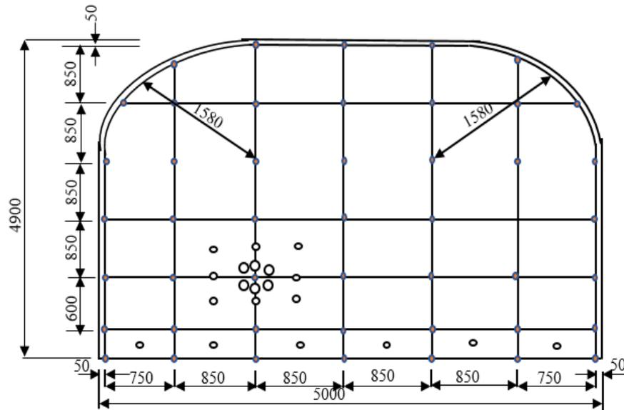
Figure 8: Drill Pattern Ore Drive at Chirano Gold Mine Limited
