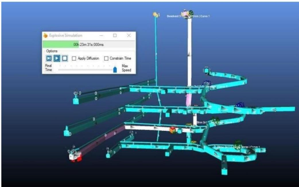
Figure 9: Single Heading Blast Simulation
