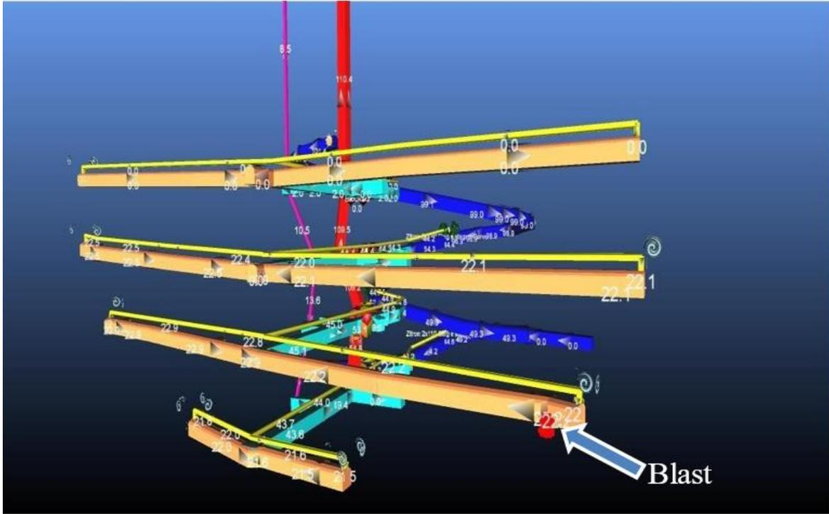
Figure 5: One Ore Drive with Single Heading Blast
