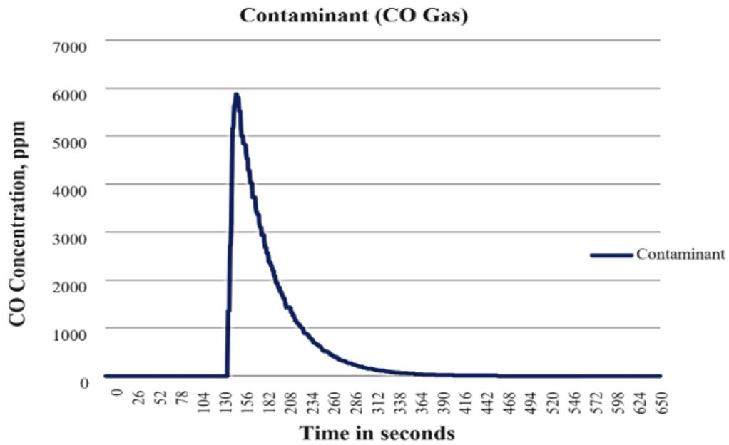
Figure 10: CO Concentration in ppm against time (seconds) (Scenario)
