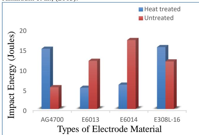
Figure 2: Impact Energy Variation of Both the Heat-Treated and Untreated Samples with Different Electrode Materials
