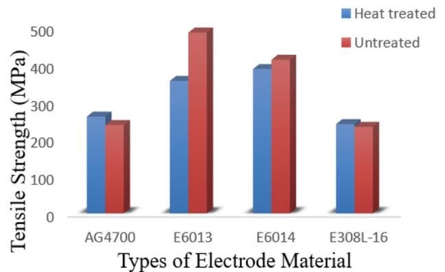
**Figure 1:** Tensile Strength Variation of Both the Heat-Treated and Untreated Samples with Different Electrode Materials
