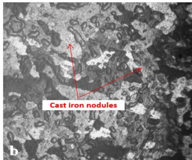
**Plate 1:** Microstructure of Mild Steel Weldment (x100) using AG4700 Electrode (a) Untreated (as-welded) (b) Heat Treated
