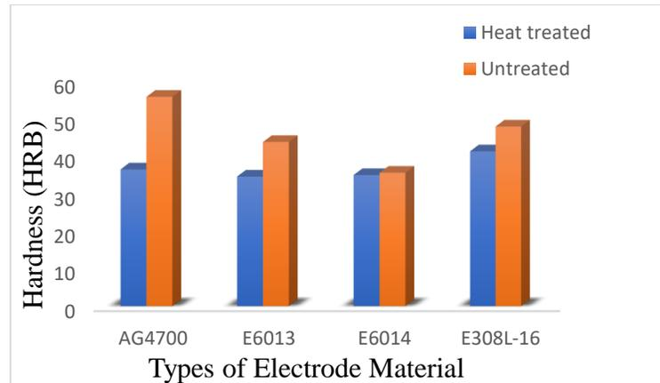
Figure 3: Hardness Variation of Both the Heat-Treated and Untreated Samples with Different Electrode Materials
