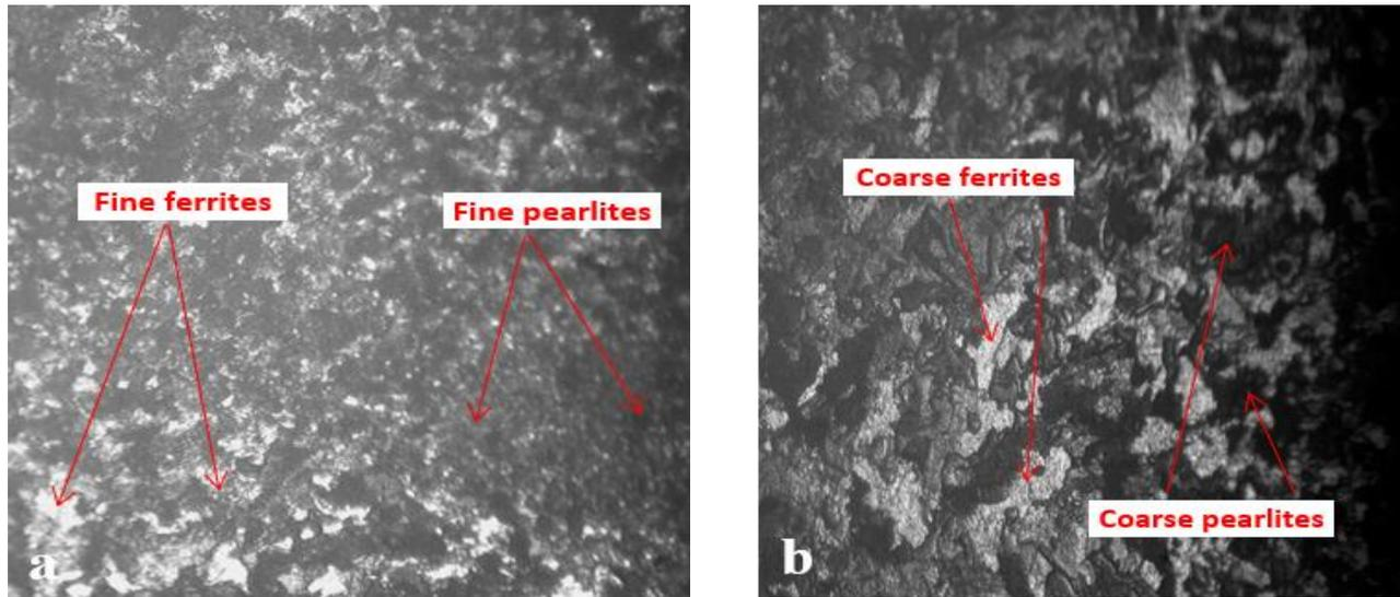
**Plate 4:** Microstructure of Mild steel weldment (x100) using E6014 electrode (a) Untreated (as-welded) (b) Heat Treated
