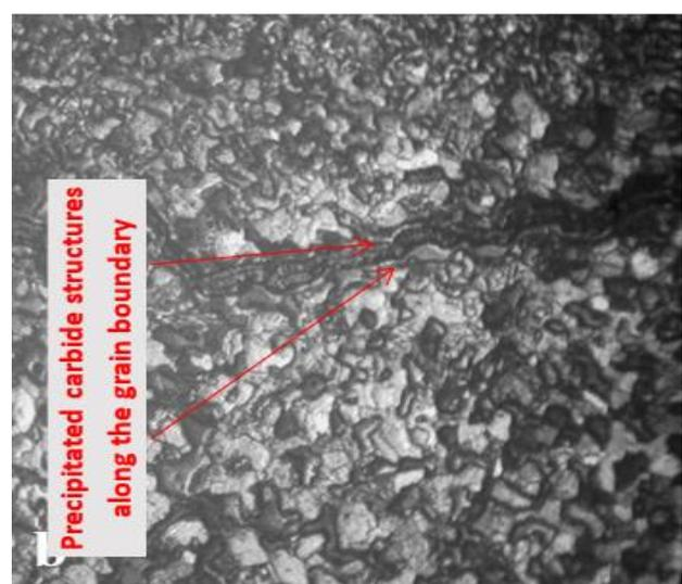
**Plate 2:** Microstructure of Mild Steel Weldment (x100) using E308L-16 Electrode (a) Untreated (as-welded) (b) Heat Treated
