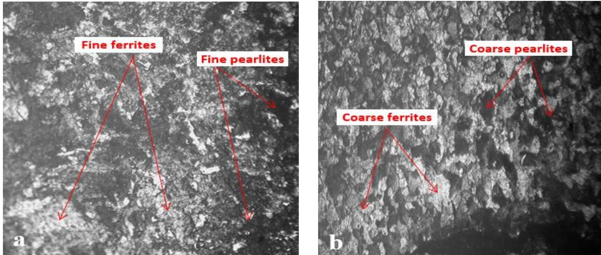
**Plate 3:** Microstructure of Mild Steel Weldment (x100) using E6013 Electrode (a) Untreated (as-welded) (b) Heat
