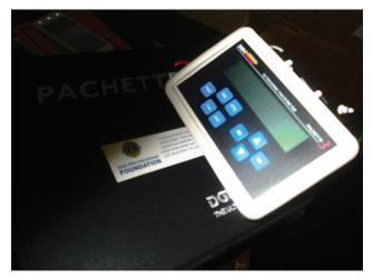
Figure 1: Ultrasonic pachymeter
