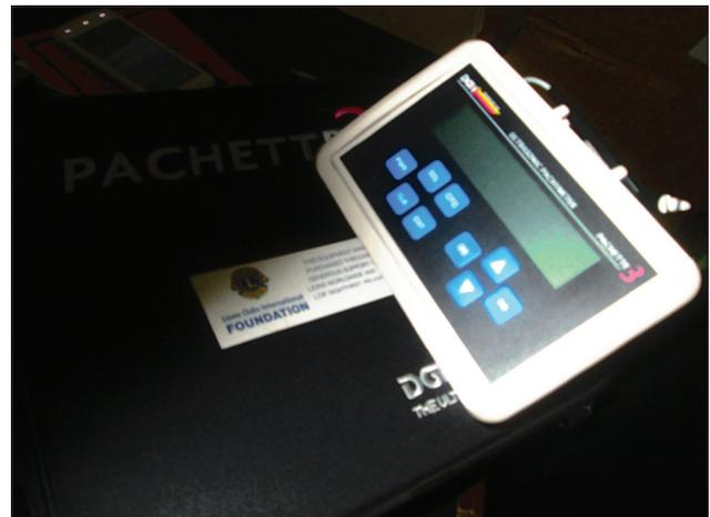
Figure 1: Ultrasonic pachymeter
