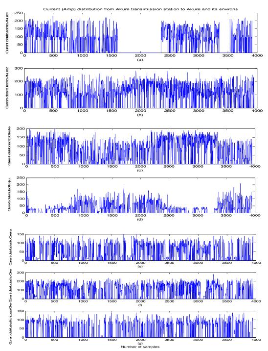
Fig. 3: Graph of total power in terms of current distributed from the 132kV Omotosho transmission station in Akure to: (a) T2B\_Akure, (b) T2C\_Akure, (c) Oba\_Ile, (d) Iju, (e) Owena, (f) Owo and (g) Igbara\_Oke.
