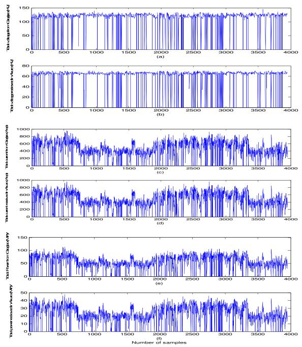
Fig. 2: Graph of total voltage (V), current (A) and power (MW) transmitted from Osogbo and received in Akure: (a) TVFO, (b) TVRA, (c) TCFO, (d) TCRA, (e) TPFO and (f) TPRA.
