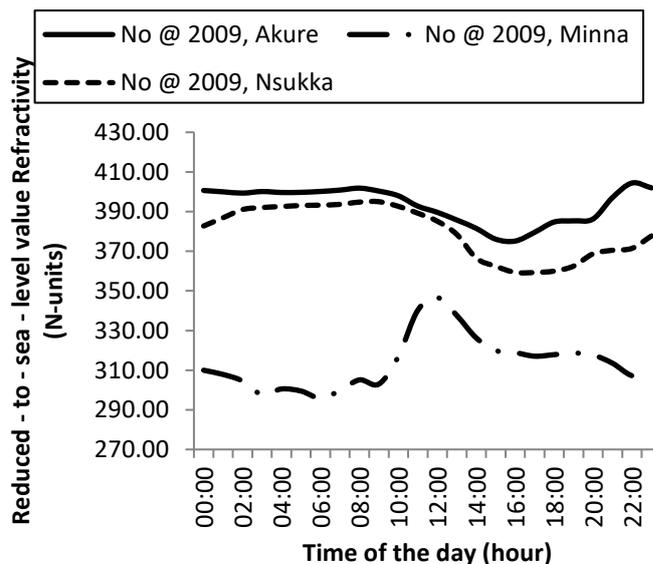
Fig. 4: Diurnal variation of reduced-to-sea-level refractivity for a typical day in the month of March 2009 across the three stations.
