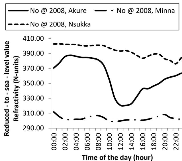
Fig. 3: Diurnal variation of reduced-to-sea-level refractivity for a typical day in the month of January 2008 across the three stations.
