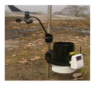
Fig. 2: The Integrated Sensor Suite (ISS) on the ground surface at a typical research site.
