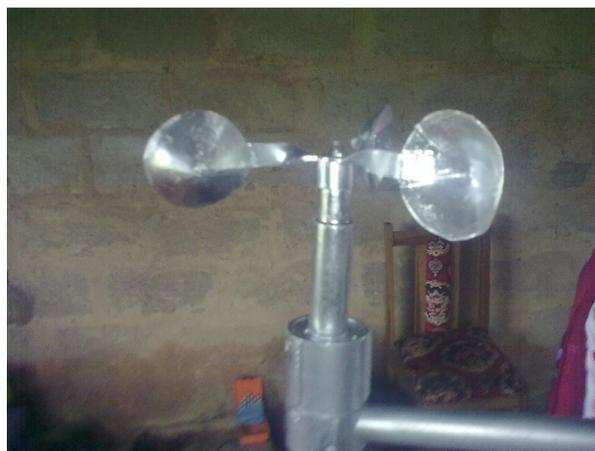
Fig. 3: Pictorial view of the constructed cup anemometer.
