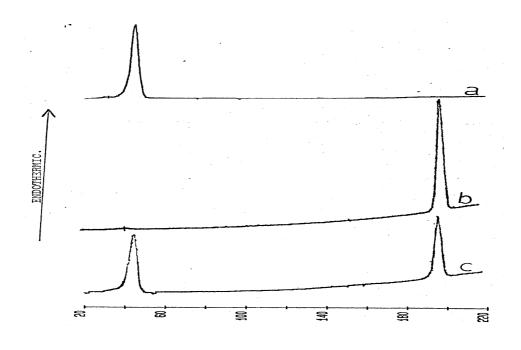
Fig. 1: DSC thermograms for dika fat and phenylpropanolamine hydrochloride. a, dika fat; b, phenylpropanolamine hydrochloride and c, 1:1 mixture of dika fat and phenylpropanolamine hydrochloride.
