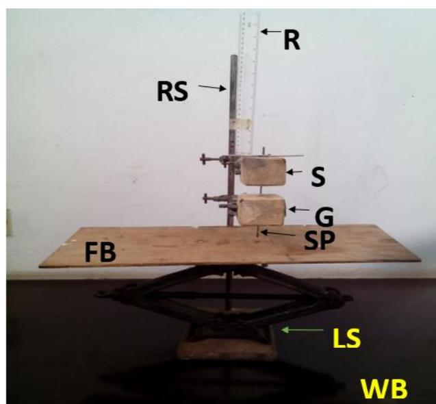
**Fig. 1:** Picture of the “weight drop” apparatus modified after Farran et al., (2014). R - Ruler, RS - Retort Stand, LS - Lever Stand, WB - Work Bench, FB - Flat Board, SP - Steinmann’s Pin, G - Guide, S – Stopper.
