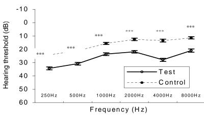
Fig. 1. Air conduction test: Audiograms of food grinding machine operators (test) and their control subjects.
