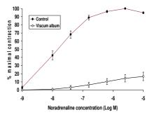
Fig.2. Concentration response curves for noradrenaline in aortic rings incubated with and without V. album (5.2mg/ml). Each point represents mean ± SEM of 6 experiments. P<0.05 at all concentrations.
