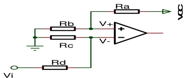
Figure 11 Comparator circuit
