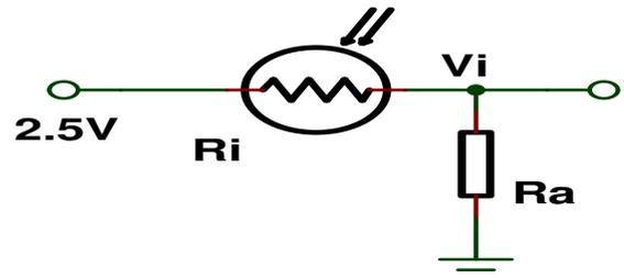
Figure 10 Voltage divider network
