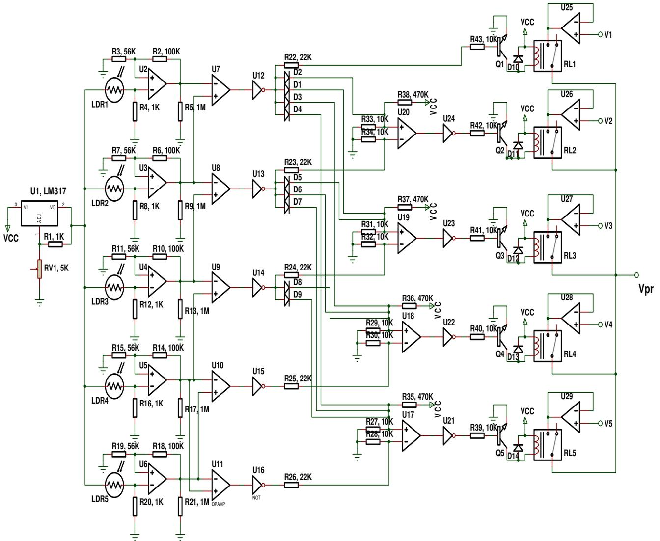
Figure 6: Priority voltage selector circuit diagram
