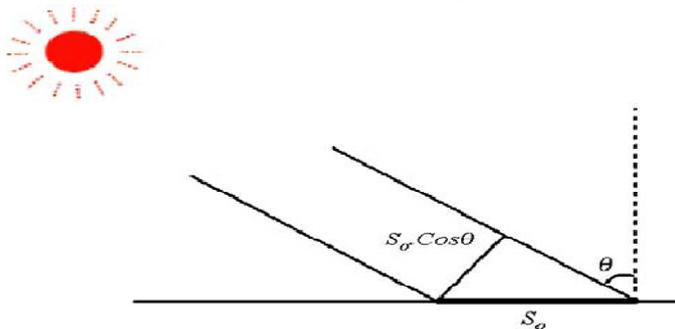
Figure 3. Angle of incidence  $u$  of the solar radiation [6]
