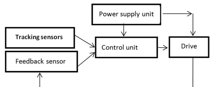
Figure 4: System block diagram
