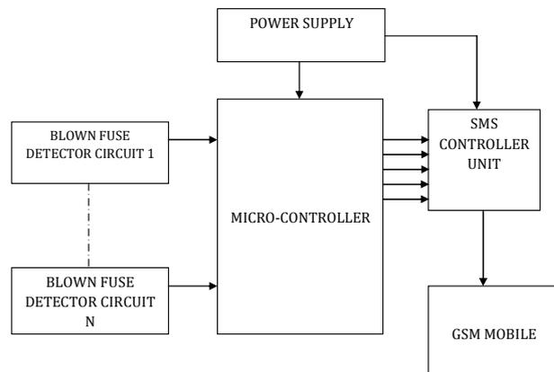
Figure 4: Block Diagram of GSM based transformer phase monitoring system
