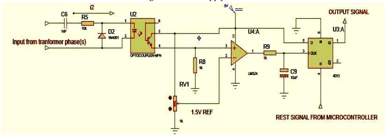
Figure 6: Blown Fuse Detector Circuit.
