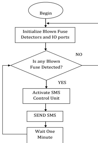
Fig. 3: Flowchart Diagram of GSM Based Transformer Monitoring System.
