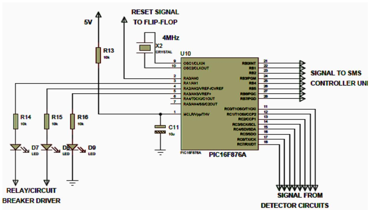
Figure 7: Systems Controller Unit.
