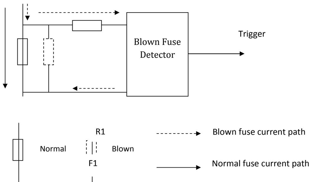
Figure 2: Descriptive Diagram of a blown fuse detector.
