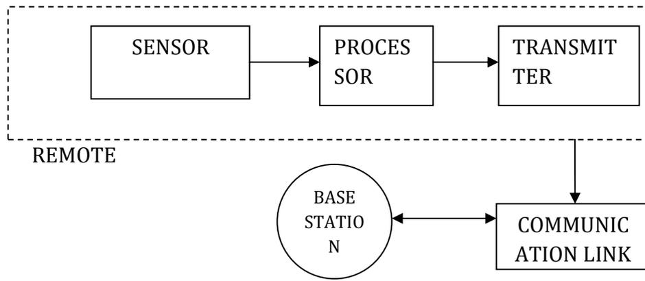
Figure 1: Basic component of a telemetry system
