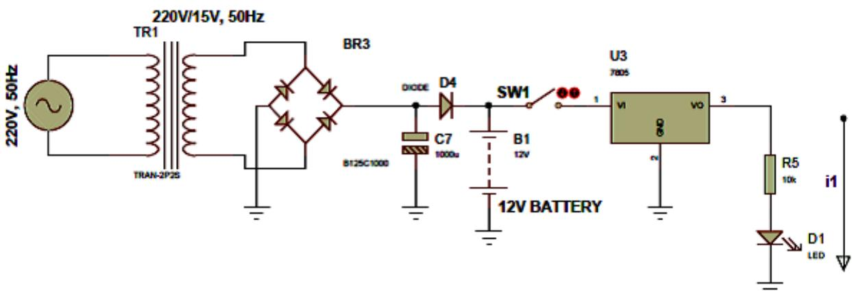
Figure 5: Power Supply Unit
