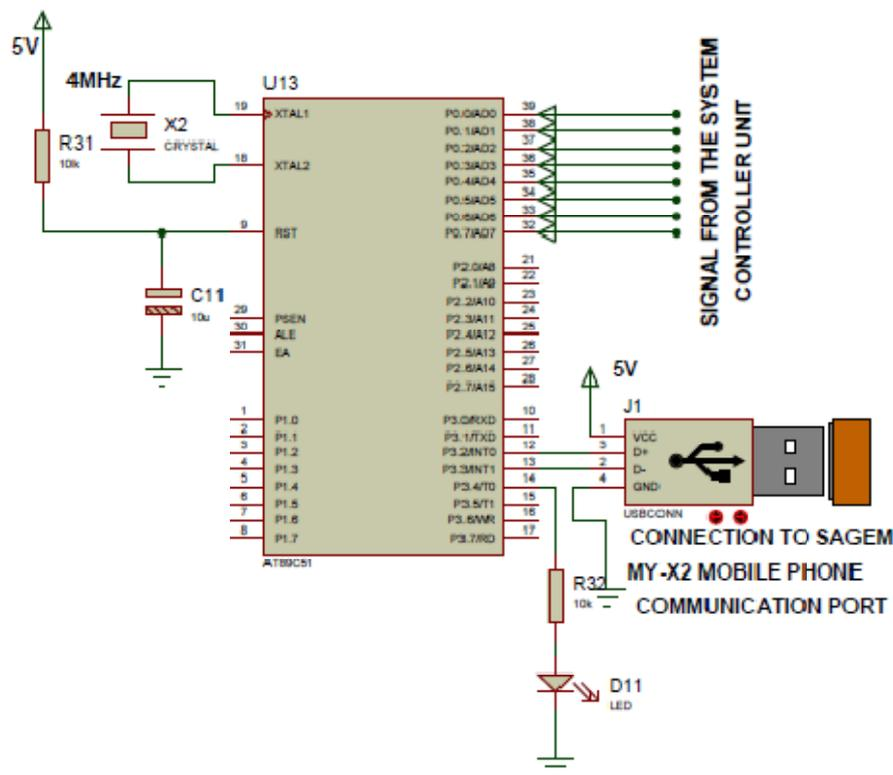
Figure 8: SMS controller Unit.
