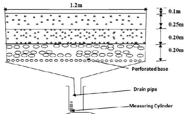
Figure 1: Schematic diagram of sand drying bed.
