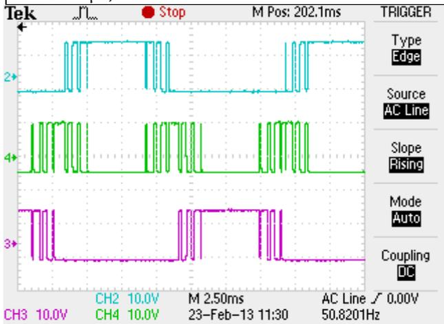
Figure 11: Experimental gate signals for phase A:  $g_1$ (channel 2),  $g_a$ (channel 3), and  $g_4$ (channel 3).
