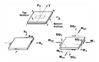
Figure 4: Notations for plate outputs
