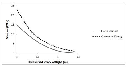
Figure 7 : Comparison of Bending Moments at Landing
