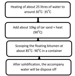
*Figure 6: Schematic diagram of extraction of bitumen from tar sand*
