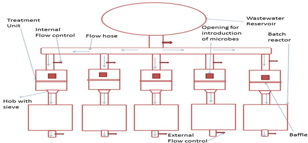
Figure A: Biosorption Pilot Treatment Plant
