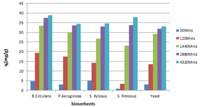
Figure 2: Variation of  $q_t$  with  $t$  (Effect of Contact Time on Biosorption of Copper)
