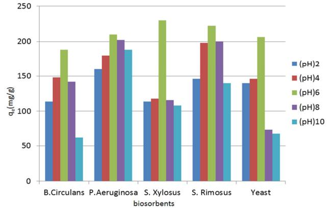
Figure 9: Variation of  $q_t$  with pH (Effect of pH of the solution on Biosorption of Manganese)
