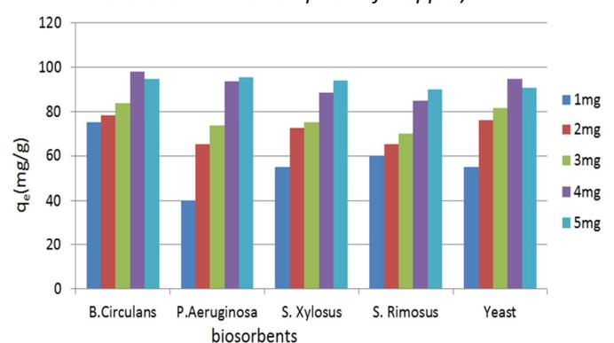
Figure 12: Variation of  $q_t$  with M (Effect of mass of biosorbent on Biosorption of Manganese)
