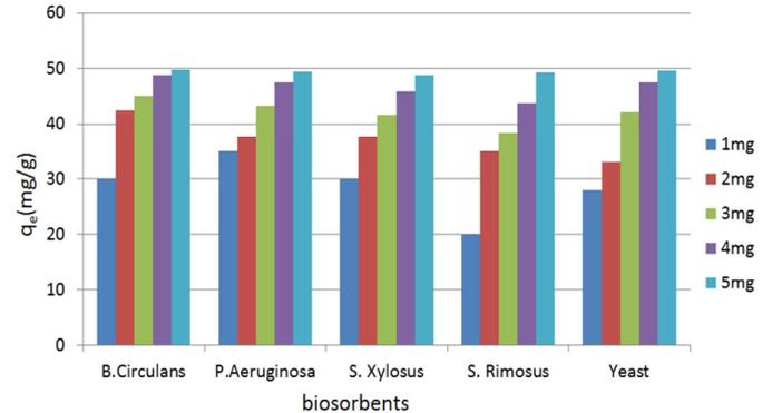
Figure 11: Variation of  $q_t$  with M (Effect of mass of biosorbent on Biosorption of Copper)
