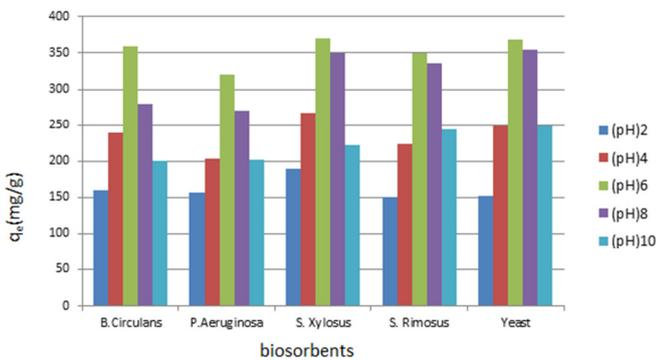
Figure 7: Variation of  $q_t$  with pH (Effect of pH of the solution on Biosorption of Zinc)
