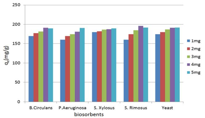
Figure 10: Variation of  $q_t$  with M (Effect of mass of biosorbent on Biosorption of Zinc)
