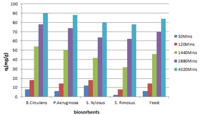
Figure 3: Variation of  $q_t$  with  $t$  (Effect of Contact Time on Biosorption of Manganese)
