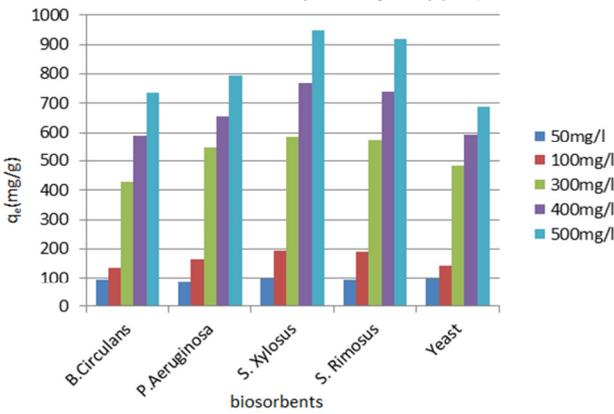
Figure 6: Variation of  $q_t$  with  $C_0$  (Effect of Initial Sorbate Conc. on Biosorption of Manganese)
