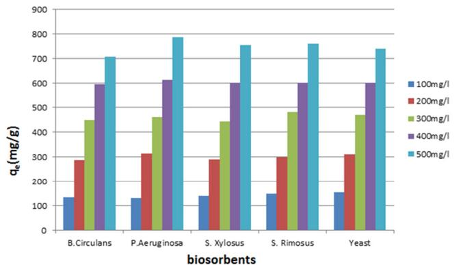
Figure 4: Variation of  $q_t$  with  $C_0$  (Effect of Initial Sorbate Concentration on Biosorption of Zinc)
