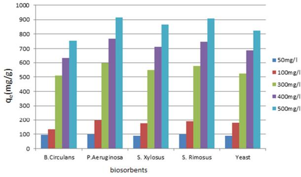
Figure 5: Variation of  $q_t$  with  $C_0$  (Effect of Initial Sorbate Conc. on Biosorption of Copper)
