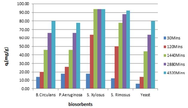
Figure 1: Variation of  $q_t$  with  $t$  (Effect of Contact Time on Biosorption of Zinc)
