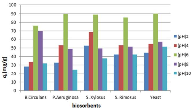
Figure 8: Variation of  $q_t$  with pH (Effect of pH of the solution on Biosorption of Coppe)r
