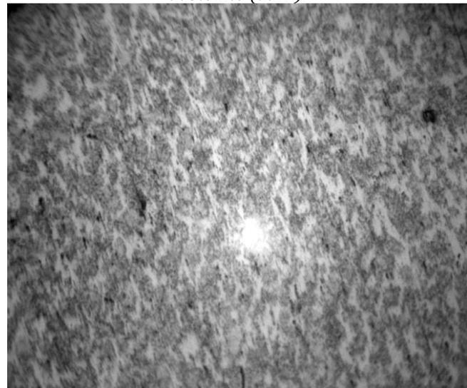
*Plate 4: Photomicrograph of B770 X400 i.e. Sample intercritically annealed at 770°C for 30 minutes. The structure reveals fine and medium size distribution of ferrite (light) matrix and martensite (gray) with little retained austenite (dark).*
