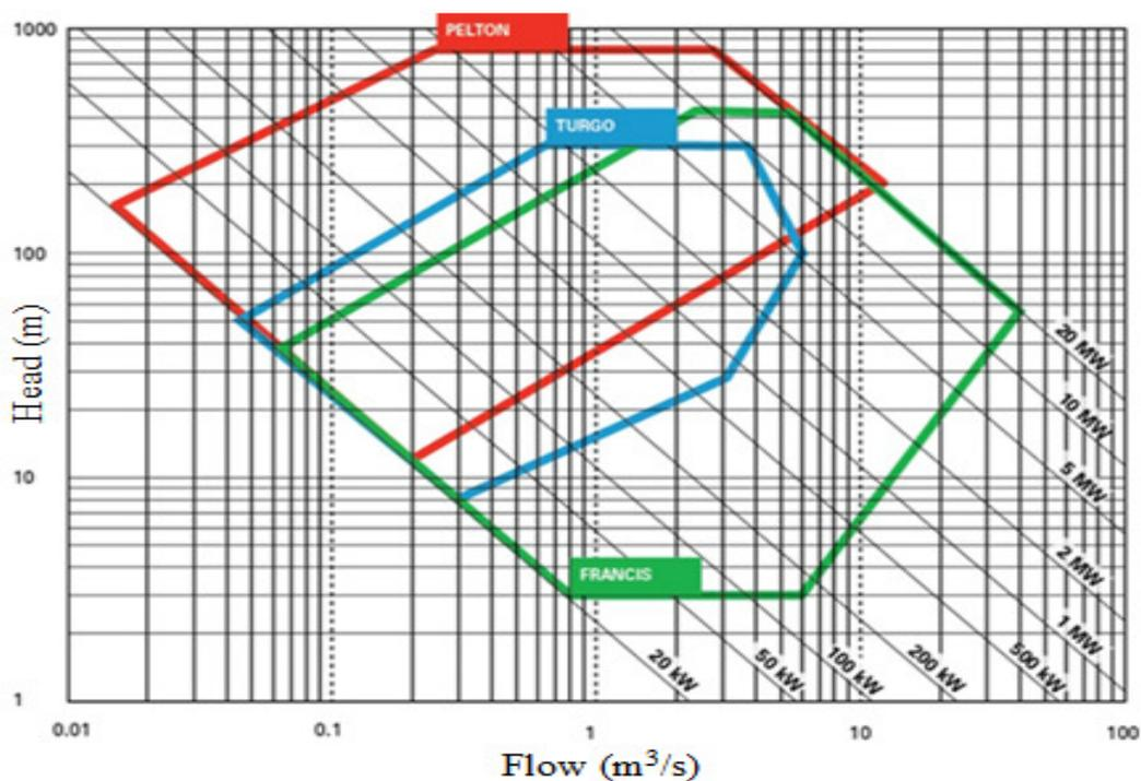
Figure 3: Turbine types and range of applications [17]
