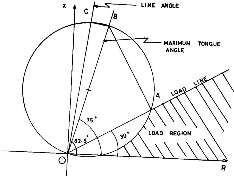
FIGURE 5: MAXIMUM RELAY REACH DUE TO LINE LOAD FOR A TORQUE ANGLE OF 75°
