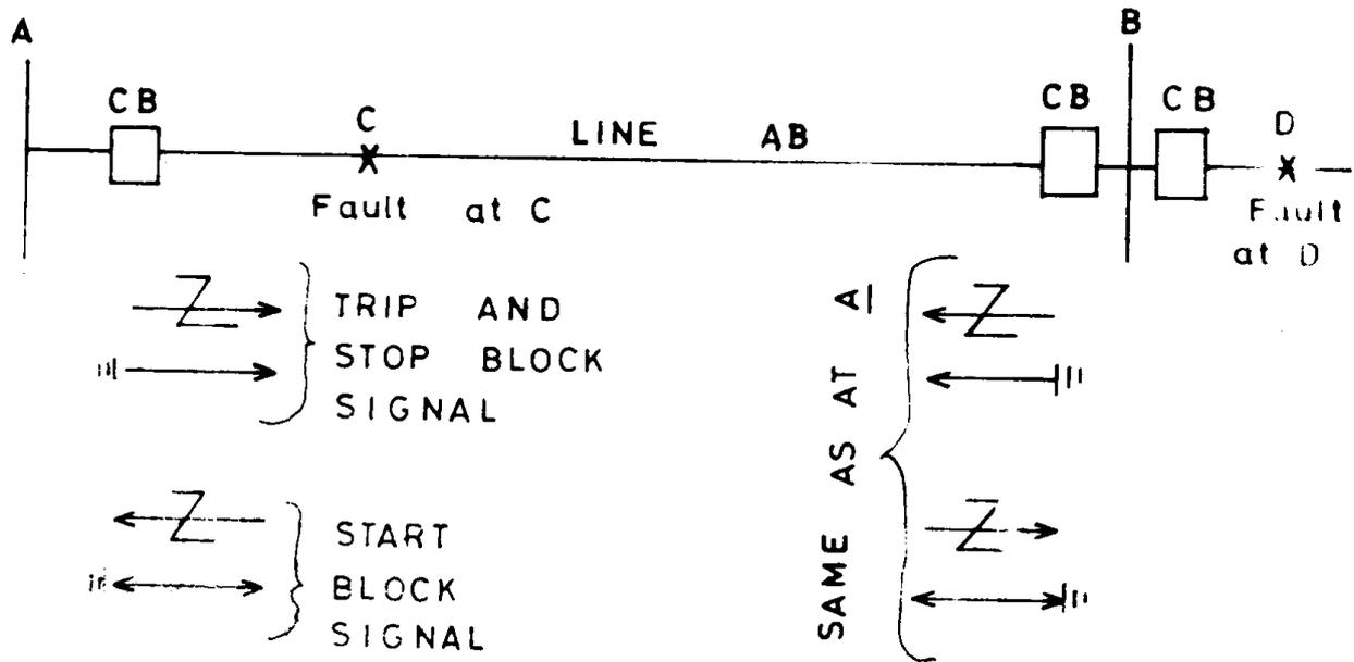
Figure 11: Directional Comparison Relaying
