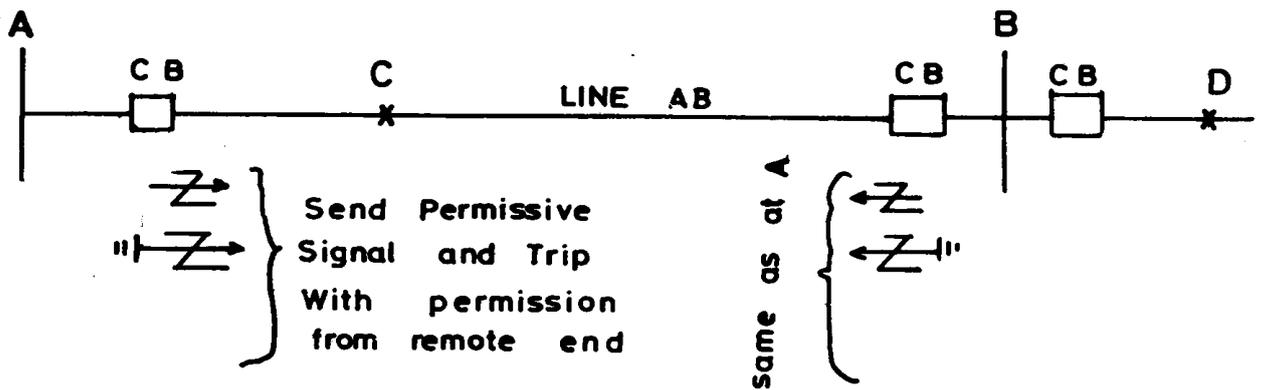
Figure 3 : PERMISSIVE OVERREACHING SCHEME
