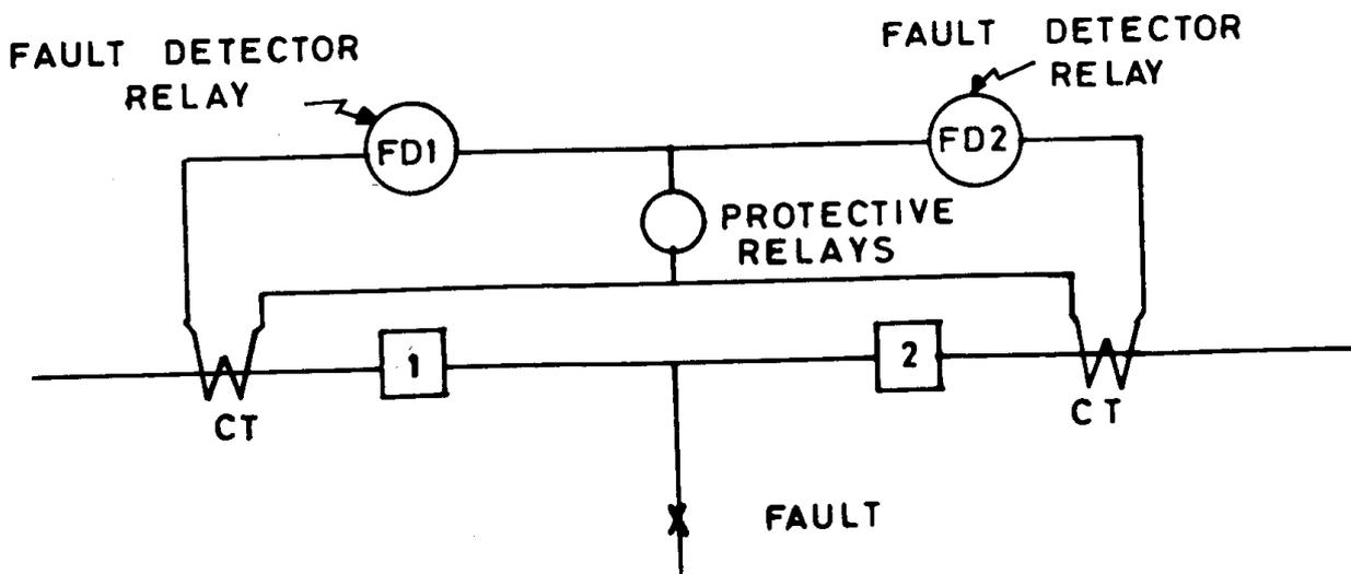
Figure 10: LBB Arrangement For The Breaker and A Half Bus Arrangement
