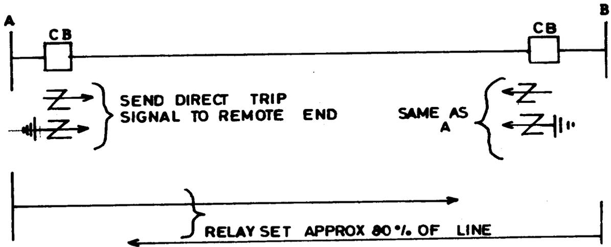
Figure 2. UNDER REACHING DIRECT TRANSFER TRIP SCHEME
