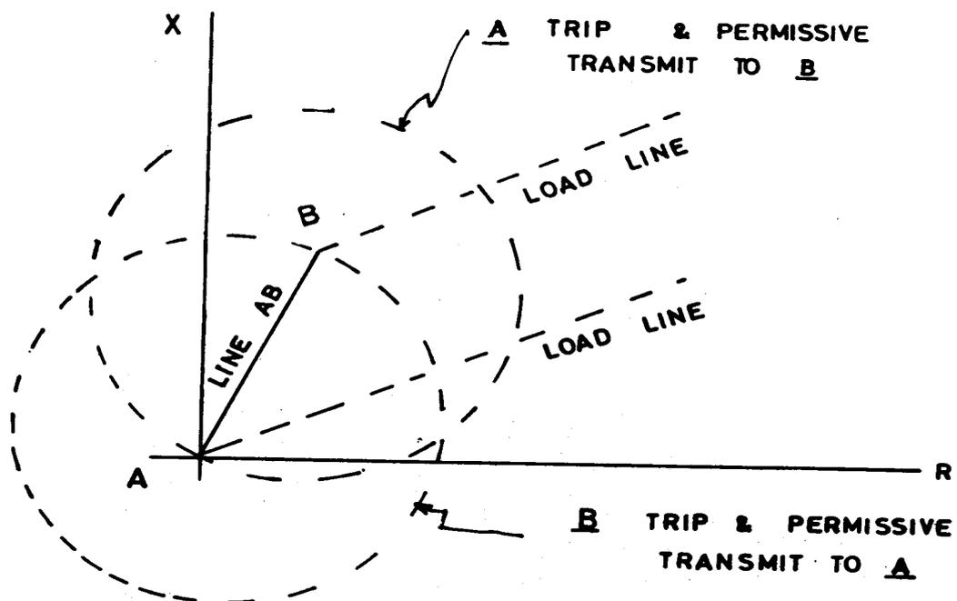
Figure 4 : TYPICAL PHASE RELAY SETTINGS FOR THE PERMISSIVE SCHEME.
