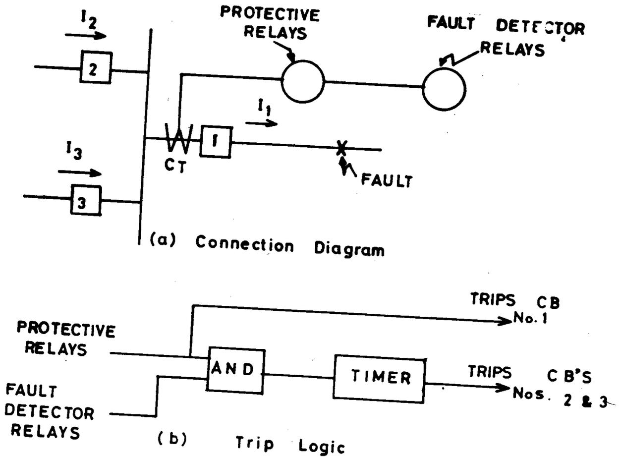
Figure 9: LBB Connection and Trip Logic For Single Bus Single Breaker Arrangement
