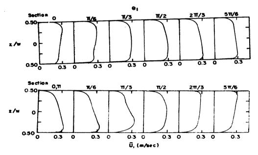
FIGURE 2. LATERAL DISTRIBUTION DEPTH-AVERAGED LONGITUDINAL VELOCITY. RUN 301/2/3
