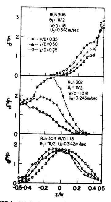
FIGURE 4 TRANSVERCE CONCENTRATION PROFILE AT VARIOUS FLOW LEVELS AND AT SECTION  $\theta_1 = TI/2$
