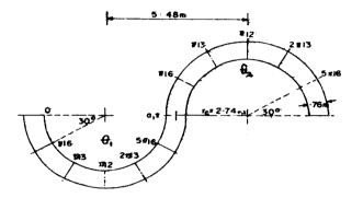
FIGURE IB SKETCH OF MEANDERING FLUME SHOWING Sections used for velocity and Concentration measurements
