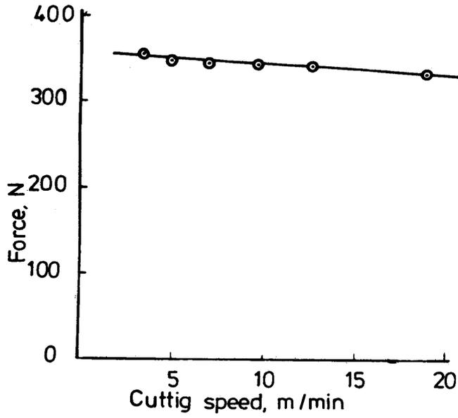
Fig. 5: Cutting force Vs Cutting speed
