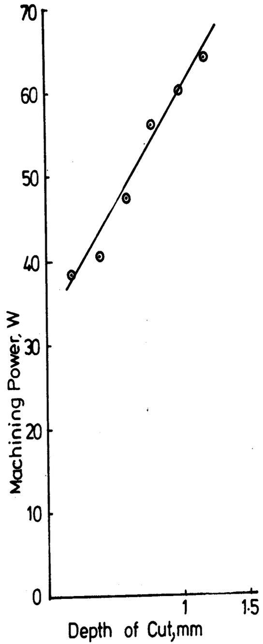
Fig. 10: Machining Power Vs Depth of cut
