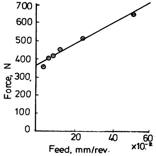
Fig. 6: Cutting force Vs feed
