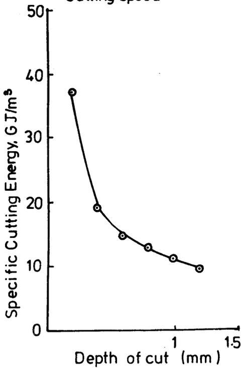
Fig 13: Specific cutting Energy Vs Depth of cut
