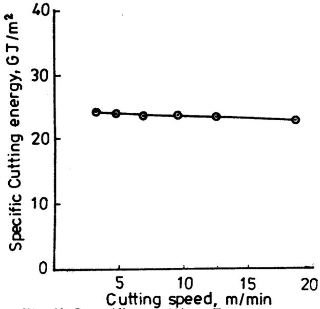
Fig. 11: Specific Cutting Energy Vs Cutting speed
