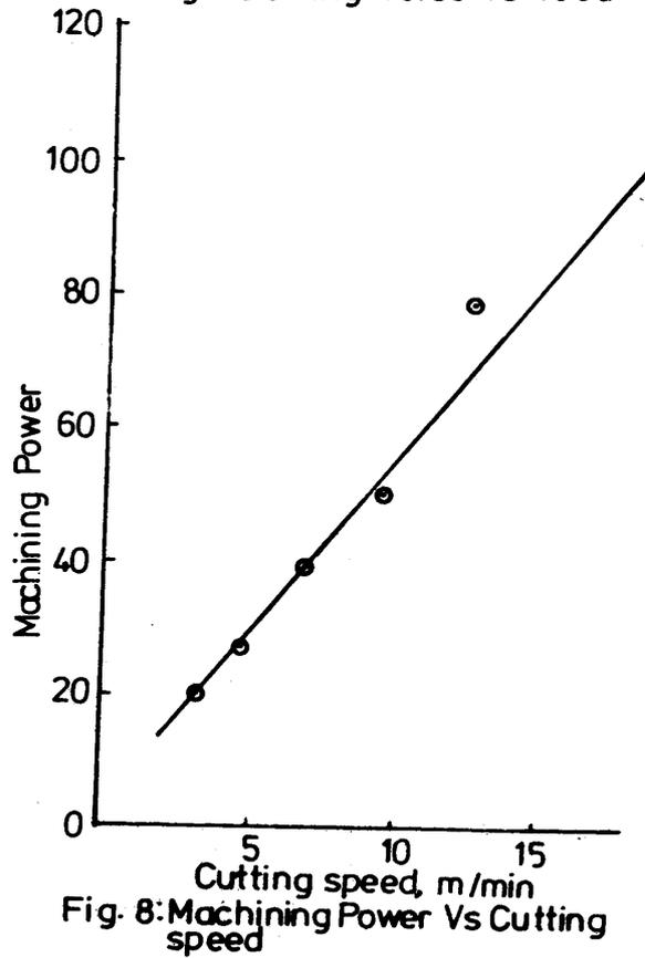
Fig. 8: Machining Power Vs Cutting speed
