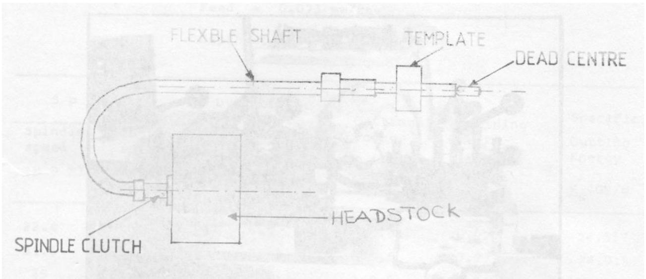
Fig.1 power from the headstock using flexible shaft drive
