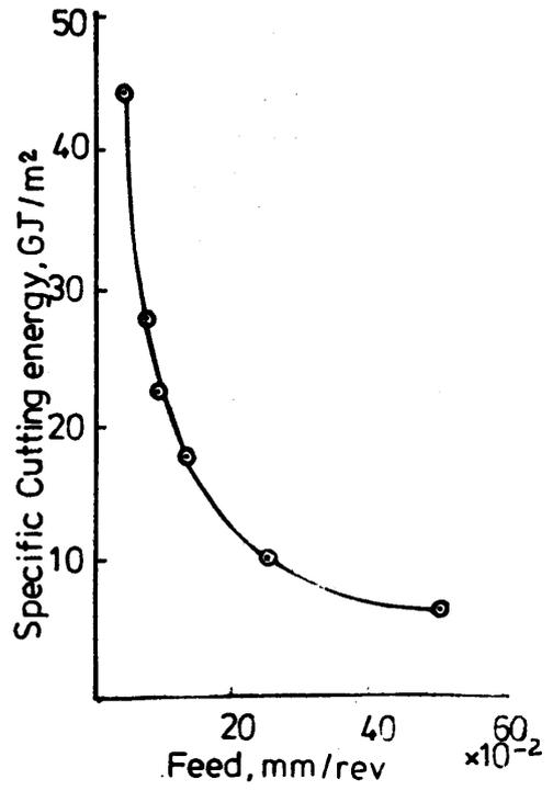
Fig. 12: Specific Cutting energy Vs feed
