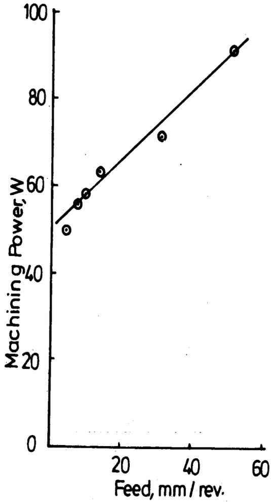
Fig. 9: Machining Power Vs Feed
