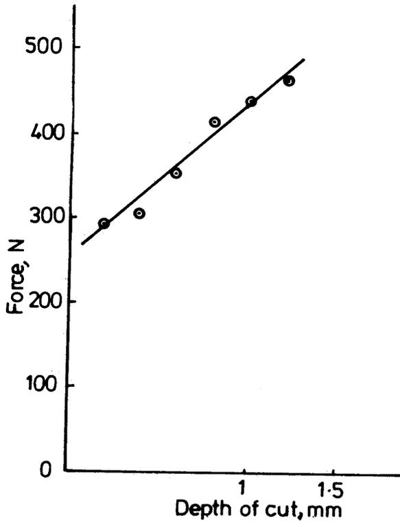
Fig. 7: Cutting force Vs Depth of cut
