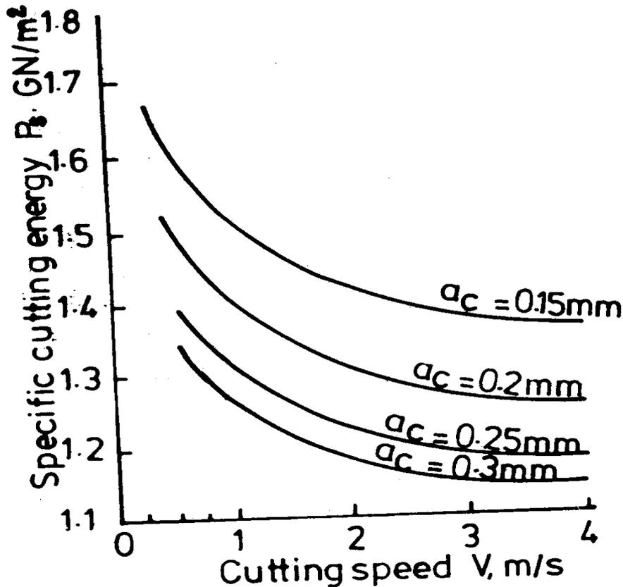
Fig.15. Effect of cutting speed and undeformed chip thickness on specific cutting energy
