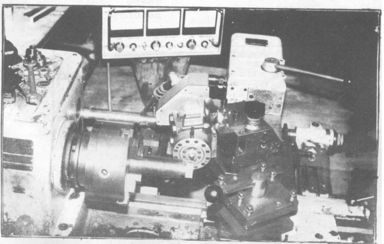
Fig. 4: Set-up for the measurement of cutting force
