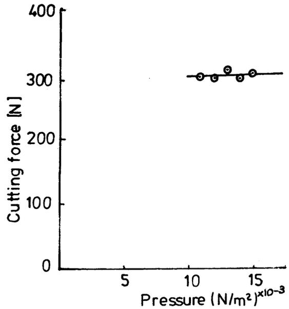
Fig. 14: Cutting force Vs follower - Template contact pressure
