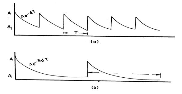
Fig. 7. Positive envelope structure of Seta data (a) at 3000 rpm (b) at 1000 rpm
