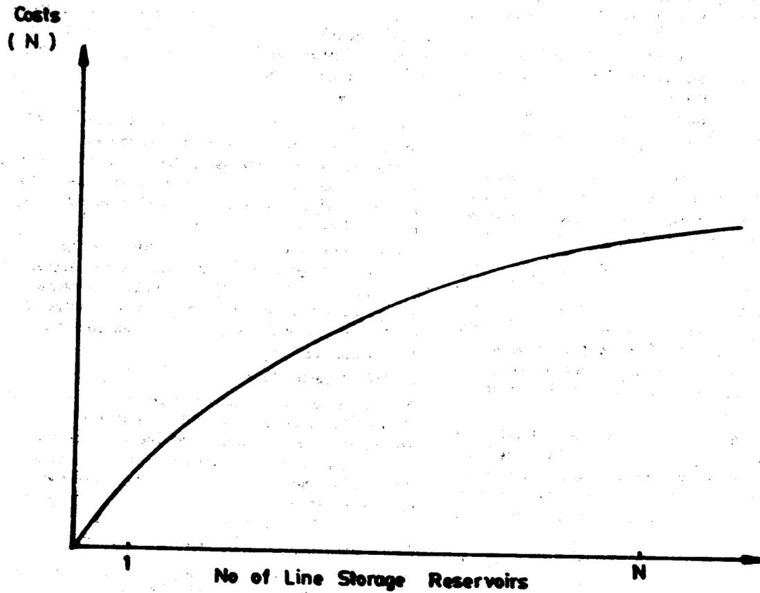
**Figure 2: COST FUNCTION FOR LINE STORAGE RESERVOIRS VS NUMBER OF LINE RESERVOIR (FOR SAME AMOUNT OF WATER STORED) (Adopted from Buhr & Woodside [9])**
