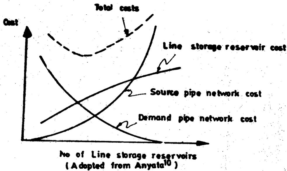
**Figure 3: THE EFFECTS OF NUMBER OF LINE RESERVOIR ON COMPONENT COST OF WATER DISTRIBUTION SYSTEME FOR THE SAME AMOUNT OF WATER STORED. (Adopted from Anyata<sup>10</sup>)**
