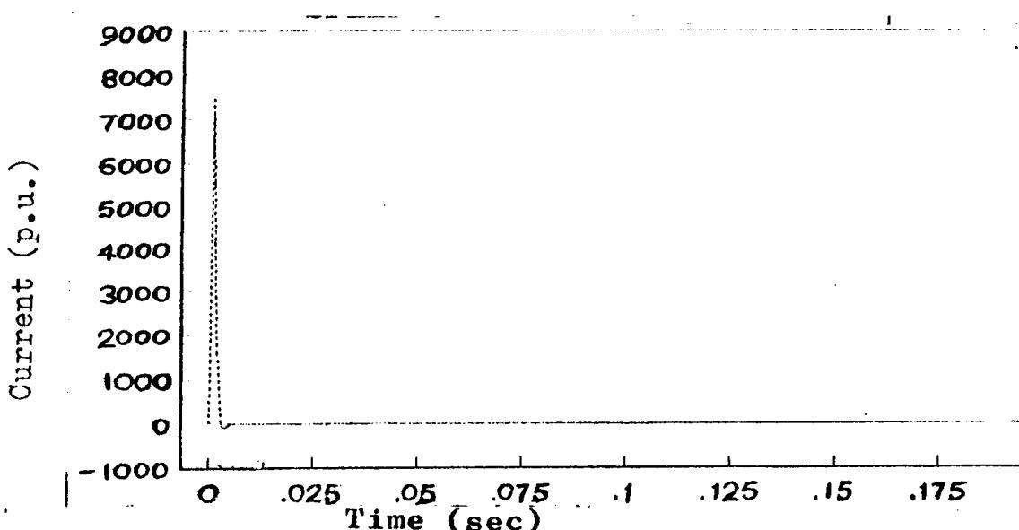
Fig. 12: Current Transient response of DCM with Proportional plus integral speed controller.
