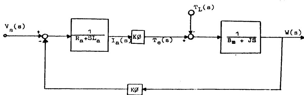
Fig. 1: Open Loop block diagram of a Separately excited d.c motor (DCM)
