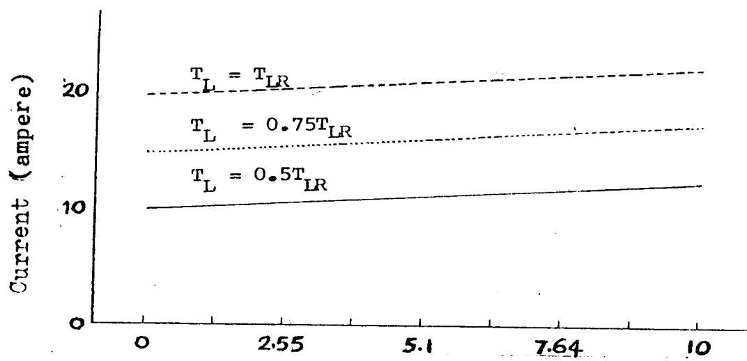
Fig. 10: Steady State Current Characteristic of DCM with Proportional Speed Controller.
