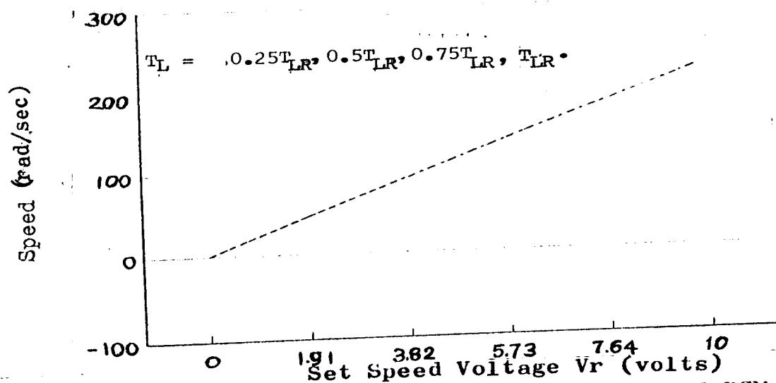
**Fig. 9:** Steady State Speed Characteristic of DCM with Proportional Speed Controller.
