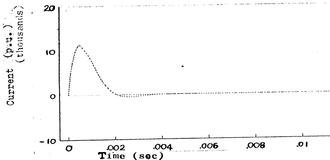
**Fig. 8:** Closed Loop Current response of DCM With Proportional Speed Controller.
