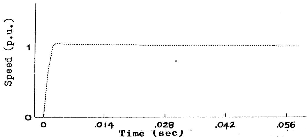
Fig. 11: Speed Transient response of DCM with Proportional plus integral Speed Controller.
