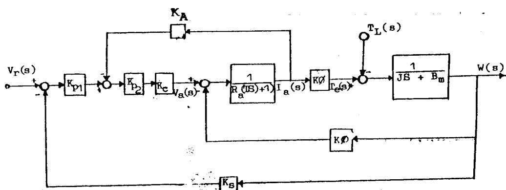
**Fig. 6:** Closed loop block diagram of DCM.
