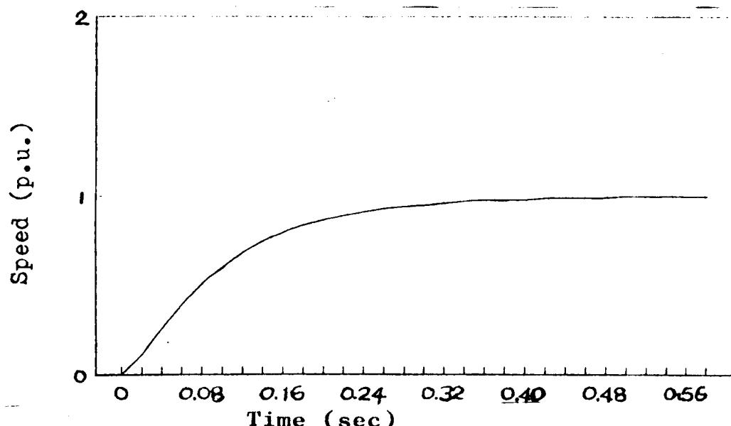
Fig. 2: Open loop transient speed response of DCM for unit step change in Voltage
