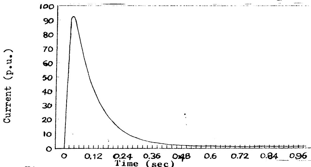
Fig. 3: Open loop transient current response of DCM for unit step change in voltage  $V_a$ .
