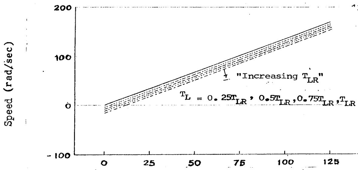
**Fig. 4:** Open loop steady state speed characteristic of DCM.
