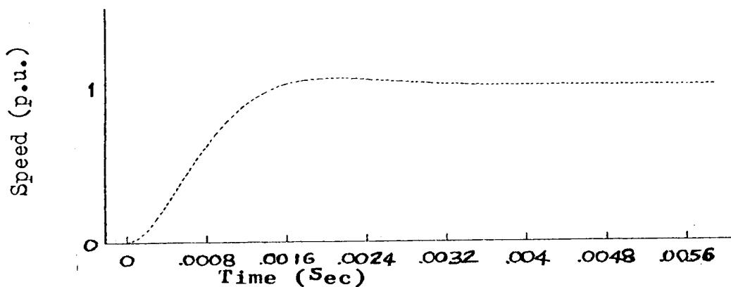
**Fig. 7:** Closed Loop Speed response of DCM With Proportional Speed Controller.
