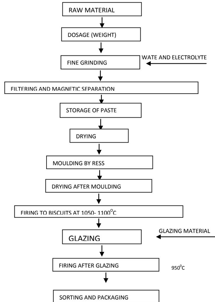
FIG.1 Flow diagram for tile production
