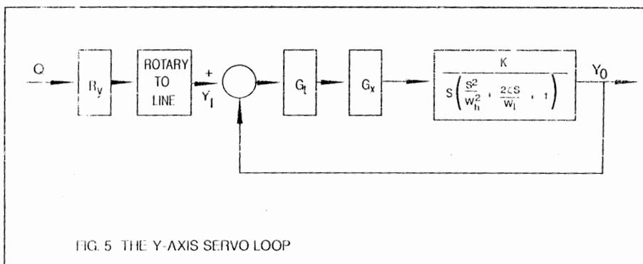
FIG. 5 THE Y-AXIS SERVO LOOP
