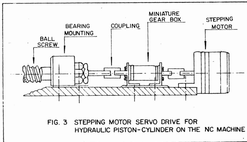
FIG. 3 STEPPING MOTOR SERVO DRIVE FOR HYDRAULIC PISTON-CYLINDER ON THE NC MACHINE
