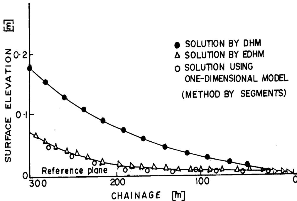
Fig.3 - Water Surface Elevation for Parallel flow in rectangular domain with uniform bed slope.
