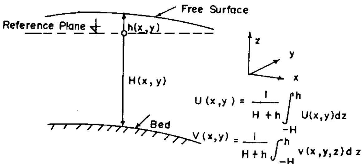
FIG. I: Definition Sketch for the System of Equations (1)-(3).
